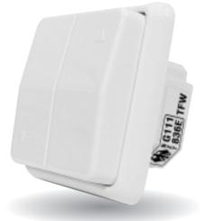
Dimmer for lights from 60 up to 500W. Suitable for halogen lighting with a wire-wound transformator. Remote control via the mains using Marmitek X-10 Commands. Memory for last dim setting. Can be combined with (designer) pulse switches. Manual control is also possible. Soft start and smooth dimming features, remembers the last dim setting. Can be regulated from 0% lighting to the desired dim setting.
